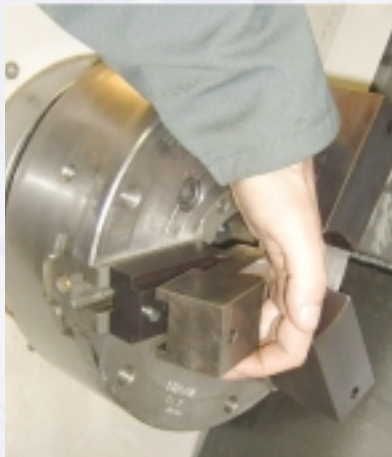
Put replacement jaw over dovetail and push jaw down over locking pin.
